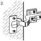
MOVE DOOR OUTWARD by turning this screw counter-clockwise
